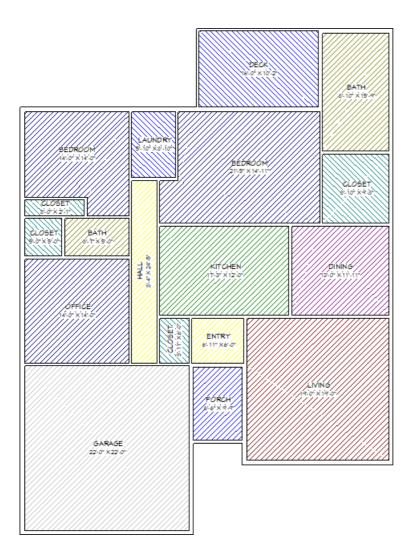
6. After the rooms are positioned and correctly sized, select **Tools> Space Planning> Build House** and on each floor level. The room boxes will be converted into walls and rooms. If Auto Rebuild Roofs is enabled, automatic roof planes will also generate.
