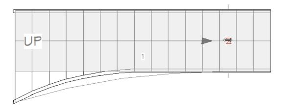
Only exposed sides of a stair section can be flared. If one side of a stair section is against a wall or wrapped, only the exposed end can be flared.
