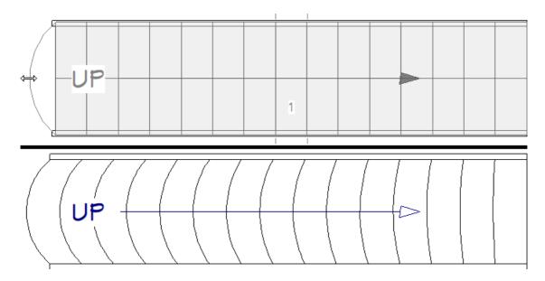
When treads are curved, all treads in the section show some degree of curvature. Treads close to the curved end have a greater curve than those at the opposite end, but both ends can be curved.
