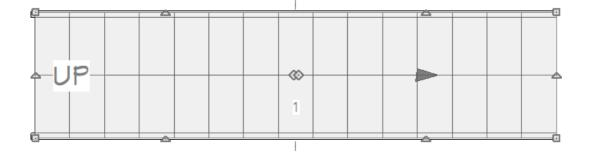
• The square handles that display at each corner of the staircase are the flare handles.
