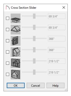
3. Check the box beside a cross section cutting plane, then either use the slider or enter a desired value using the text field.
