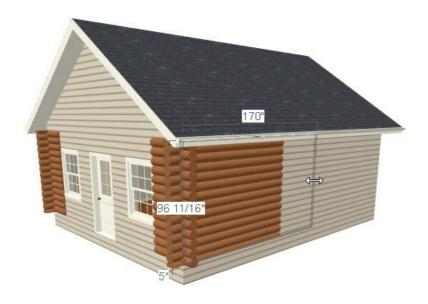
While in a 3D view, select the facade and use the edit handles that display to stretch it so that it covers the entire wall.
