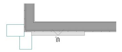
You can click anywhere in floor plan view to place it; however, if you click close to the exterior of a wall, it will automatically snap onto the wall's surface with the flat side facing inward and the log facade facing outward.
