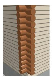
7. Repeat this process for the remaining corners of the structure, making sure that 8-13 Full and 8-13 Half corners do not share the same wall, but are always around the corner from one another.
