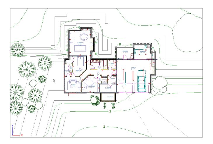
3. Next, select **Terrain> Terrain Wall and Curb> Straight Retaining Wall**, then click and drag to create retaining walls out from the garage.
